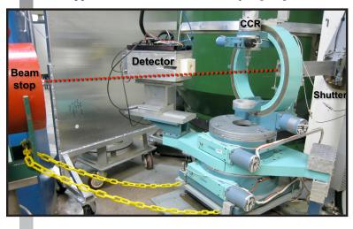
reflection from planes of the <011> zone ensures sharp diffraction peaks in specified ranges of detector angles by control of the horizontal radius of curvature. Any plane from the <011> zone can be set in Bragg position, but only the (331), (220) with (440), and (111) with (333) reflections are of practical interest. For the fixed monochromator angle of 48°, these reflections provide principal incident
