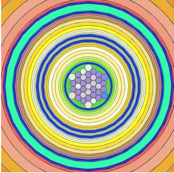
Fig. 7. Cross section of SCALE model across the flux trap and fuel elements.
