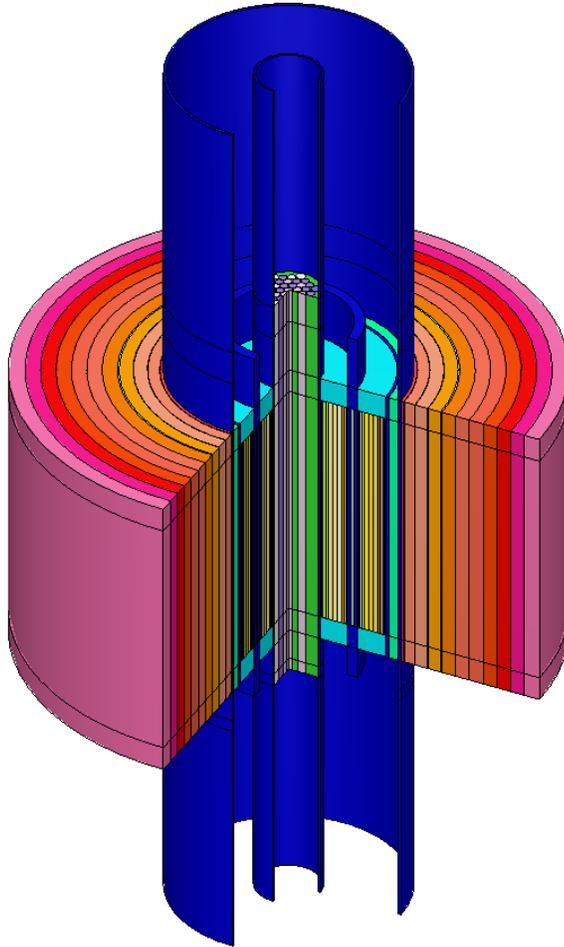
Fig. 14. Isometric view of the HFIR SCALE model.
