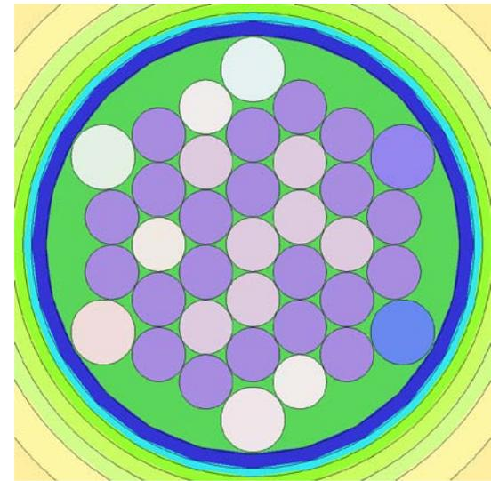
Fig. 5. Cross section of SCALE model across the flux trap.
