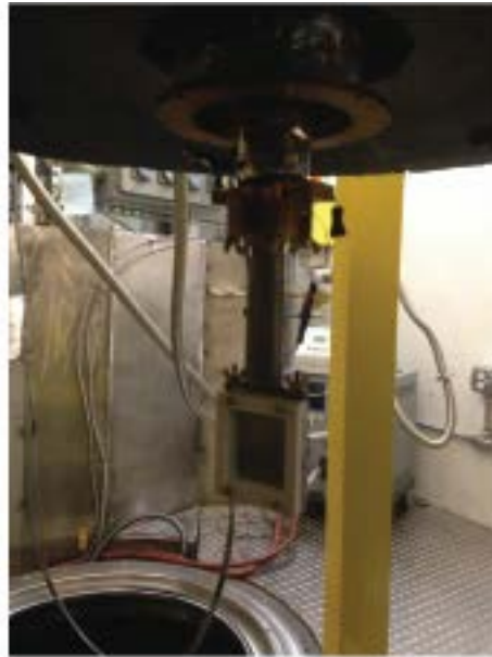
Figure 14 Flat cell schematic (left) and installed on CCR-13 (right) with a boron nitride mask.
