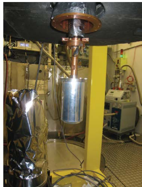
Figure 12 Dimensions for the "soda" can (left) and one installed on the bottom of CCR-13. The foil on the left side of the photo is the heat shield commonly used on CCR-13
