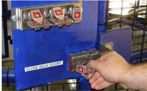
Figure 5. Rotating Ib key counter-clockwise for removal from door lock
