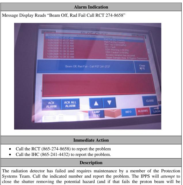
close the shutter removing the potential hazard (and if that fails the proton beam will be tripped). Do not attempt to open the shutter until the condition causing the radiation monitor to fail is corrected, and granted approval by the Protection Systems Team Leader or designee.
