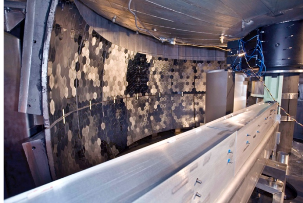
Figure 2. Inside the BASIS tank, view from the open tank door. Shown are the incident beam guide (enclosed in the shielding) and the crystal analyzer panels.
