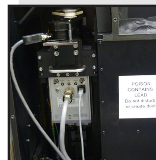
Detector housing for the CCD camera lens, mirror, and scintillator.
