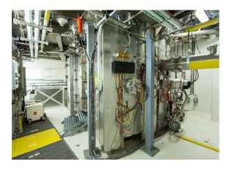
discrimination by modulating the incident beam with a statistical chopper. At the same time, CORELLI can host complex sample environments because of a large sample scattering vessel. A complete data set is collected in 30 to 90 individual measurements, depending on the crystal symmetry, scattering strength, sample size and resolution needed, resulting in an average experiment time of 2 days.
