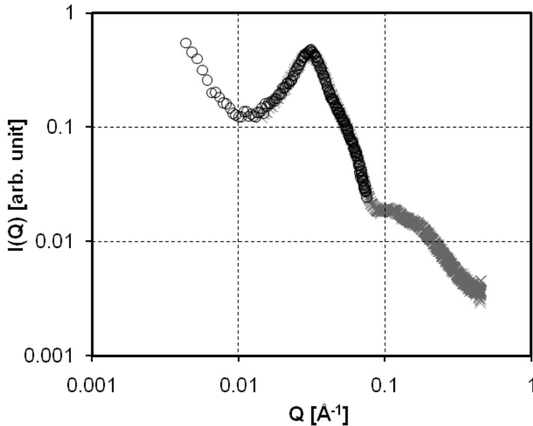
FIG 2. Scattering data of a dendrimer sample [10] processed to  $I(Q)$  using the *fatcat* software. The sample was measured in the frame-skipping mode with frames at 2-5.4Å and 8.9-12.3Å and the sample-to-detector distance of 5m. Data from the two frames are reduced separately to illustrate their  $Q$ -ranges. The overlapping grey crosses are from the frame at 2-5.4Å and the black circles are from 8.9-12.3Å. Their region of overlap lies between  $Q \sim 0.02-0.08 \text{Å}^{-1}$ .
