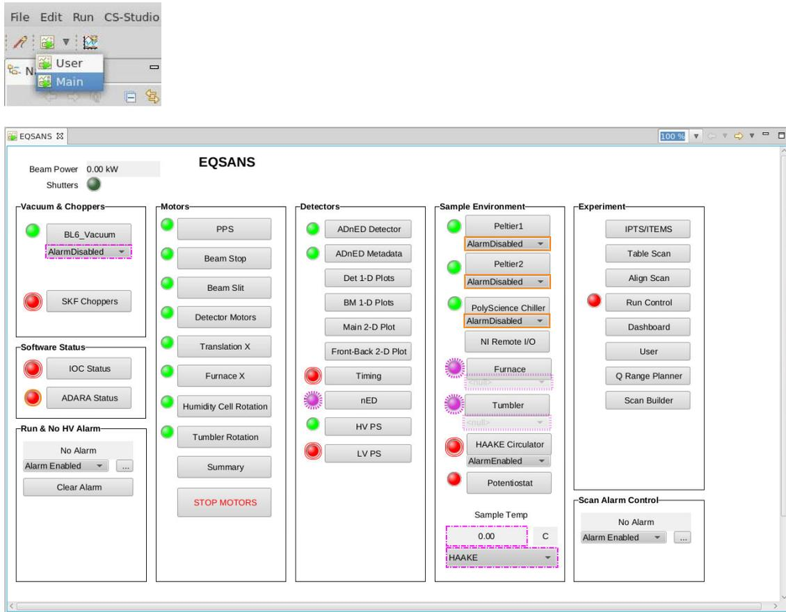
Lights indicate the state of the instrument controls: green = OK, red = error, purple = disconnected.
