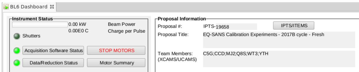
The SNS beam status is listed at the top of the **BL6 Dashboard** tab in the **Instrument Status** box. The Beam Power (kW) and Charge per Pulse (C) are given. Proposal details (e.g. IPTS #) also are listed at the top in the **Proposal Information** box.
