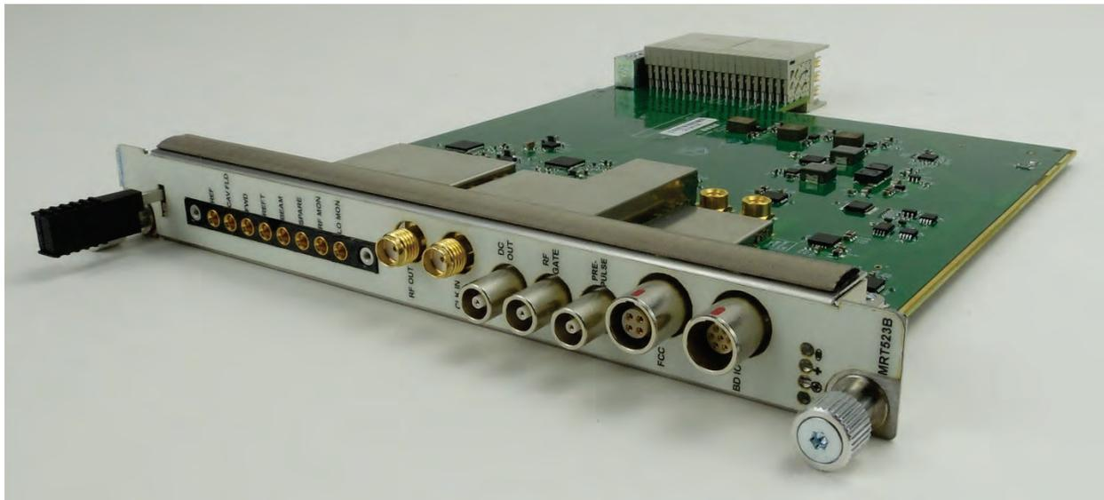
**Figure 4.11. Field control module-II rear transition module.**
