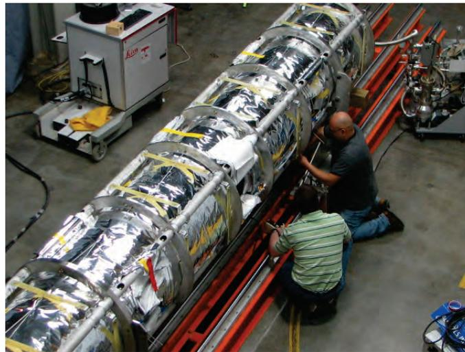
**Figure 3.12. Cryomodule cold mass assembly.**
