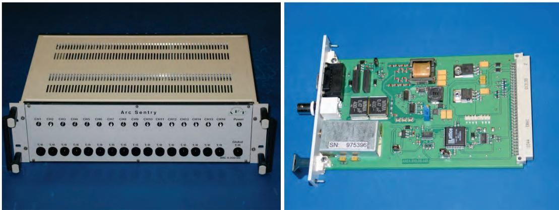
Figure 4.13. Advanced Ferrite Technology arc detector system.
