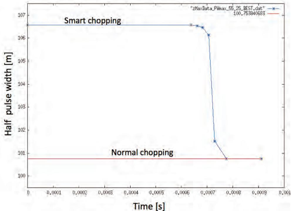
**Figure 2.1.** Example pattern width variation over the ring injection cycle leading to a clean extraction gap with 5% higher charge per pulse. Blue line: pattern width variation that results in higher beam charge. Red line: example of constant pattern width in use today.
