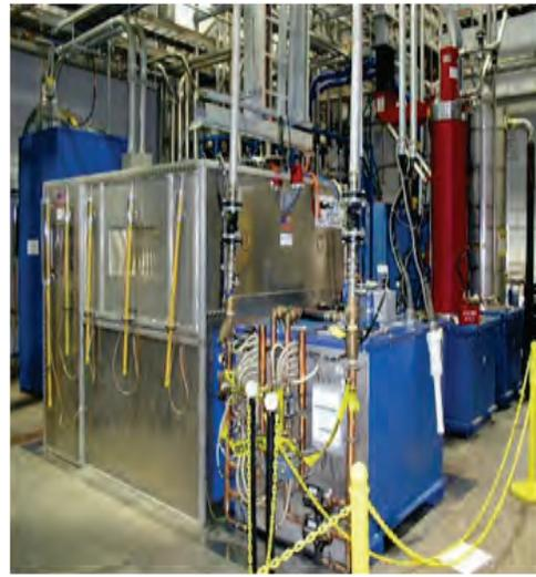
Safety enclosure and oil-filled modulator tank
