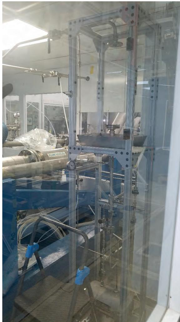
**Figure 8.33. Filter media test stand installed inside TTF. Note the test section has been removed.**
