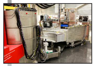
optics, plus a position-sensitive detector bank, leads to a highly flexible instrument in which the energy and wave vector resolution can be independently varied by nearly an order of magnitude. Either full or partial neutron polarization analysis can be deployed on HYSPEC. This is accomplished by using a Heusler crystal array to polarize the incident beam and a supermirror wide-angle polarization analyzer for the scattered beam.
