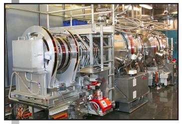
superconducting technology with high-magnetic-field homogeneity, state-of-the-art field correction elements, novel polarizing benders and location at the Spallation Neutron Source, the SNS-NSE spectrometer achieves high data collection efficiency, allowing nearly gapless coverage of a broad wave-vector time range with only a few scattering angle settings. For a maximum wavelength span of 2 Å  $< \lambda < 17$  Å, the SNS-NSE spectrometer yields an unprecedented dynamical range
