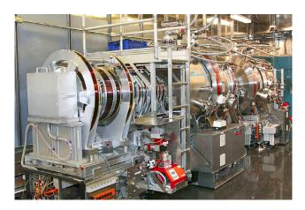
Routinely, the NSE spectrometer at SNS operates over a wavelength span of 5 Å <  $\lambda$  < 11 Å, in two operation modes, using a simultaneous wavelength frame of 2.4 Å–3.1 Å, and delivers Fourier times of over 1 ps <  $\tau$  < 130 ns for a wide q range of 0.05 Å–2.5 Å. Performance of the SNS-NSE is also extended by a positionsensitive, two-dimensional <sup>3</sup>He detector with a broad detection region.
