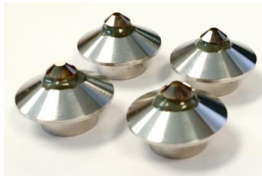
6 mm conical CVD anvils inside steel seats.
