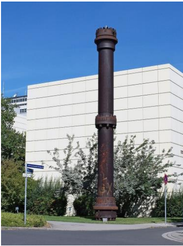
A historical (1921) high-pressure steel reactor at KIT, Germany
