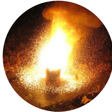
Thermite reaction: Al-Fe 2 O 3
