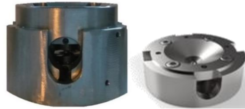
BX90 & Diacell120 with Boehler-Almax seats and diamonds Single-crystal X-ray Diffraction Brillouin Spectroscopy or Non-crystalline X-ray Diffraction (PDF)
