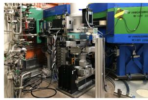
resolution can be controlled with the premonochromator collimation ( $\alpha_1$ ), which is open, 60' effective, and via three choices of presample collimation ( $\alpha_2 = 16$ , 21, or 31'). The instrument can operate in polarized mode with the use of a polarizing supermirror V-cavity optimized for the 2.41 Å wave.
