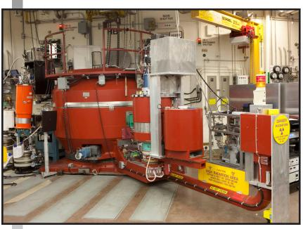
space. The sample goniometers and a full software implementation of the three-dimensional sample orientation matrix allow measurements outside the traditional singlescattering plane. The unique capability of HB-1 is the polarized configuration for studies of excitations, phase transitions, structures, and density distributions in magnetic materials.
