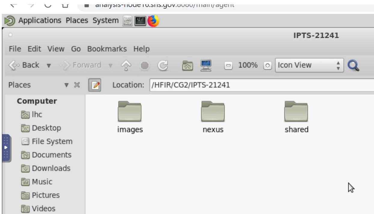
Go to the /HFIR/CG2/your IPTS number folder. The raw data are saved in nexus folder. The reduced data are saved in shared/reduction/3\_configs/1D and 2D folders.
