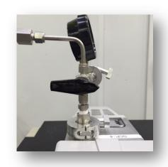
30. It is now safe to power off the vacuum pump. Remove the vacuum pumping line and helium gas cylinder. Ensure the helium gas cylinder regulator isolation valve is in the closed position.
