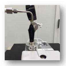
10. Disconnect the sample stick sensor cable from the sample stick.
