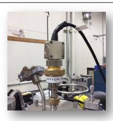
11. Loosen screws (or clamp) from sample stick flange (or flange blank), but **DO NOT** remove completely. If the sample stick (or flange blank) move freely, the space is full of helium gas, has vented off excess pressure, and it is safe to remove screws (or clamp).
