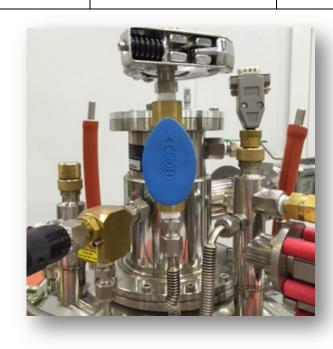
9. Vent the sample space with helium gas by turning the black 3-way valve on the vacuum pump to the up position. Wait for the vacuum gauge to read 1000 mbar.
