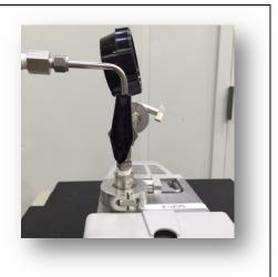
7. Vent the vacuum pumping line with helium gas by turning the black 3way valve to the up position. When the gauge on the pump indicates a pressure of 1000 mbar, begin pumping on the vacuum pumping line by turning the black 3-way valve to the down position. Repeat this step 2 times.
