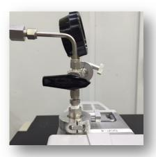
28. Immediately close the blue 3-way valve on the sample space by turning to the horizontal position.
