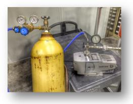
6. Power on the vacuum pump, and begin pumping on the vacuum pumping line by turning the black 3-way valve on the vacuum pump to the down position.
