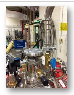
15. Begin pumping on the sample space by turning the black 3way valve on the vacuum pump to the down position.
