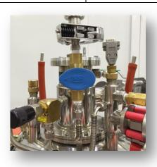
29. Vent the vacuum pumping line by turning the black 3-way valve to the up position until the vacuum gauge reads 1000 mbar. Once the line is vented, close the black 3-way valve by turning to the horizontal position.
