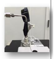
8. With the vacuum pumping line under vacuum, indicated by a pressure of zero on the vacuum gauge, and the black 3-way valve in the down position, open V-6 by turning the blue 3-way valve to the up position. You are now pumping on the sample space.
