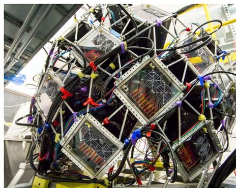
sampling of Braggpeaks in specific directions. Currently, TOPAZ has 25 of 48 detector ports populated with Anger camera modules covering a scattering angle between  $20^\circ$  and  $160^\circ$  in  $2\theta$ , matching 3.2 sr in solid angle coverage. A full dataset for structure analysis can be collected with 4 to 25 settings with an exposure time of about 0.5–5 hours each, depending on the crystal symmetry, sample scattering strength, and crystal size.
