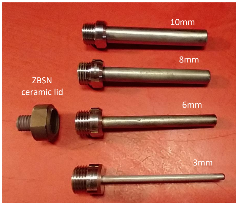
Figure 2. Can assembly for MICAS Vacuum Furnace.
