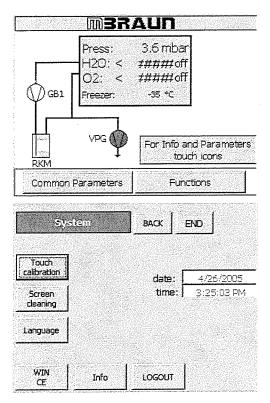
All system functions are locked out for 30 seconds while a screen with a timer bar is displayed to allow the user to clean the screen without interfering with system processes.
