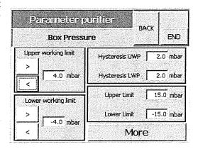
Enter the desired limit and touch the button to return to the Box pressure screen.
