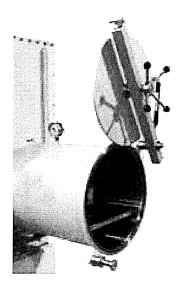
Close the outer door by pulling it down until groove at the end of the arm rests on the spindle.
