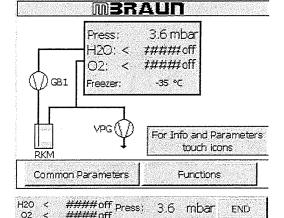
Touch the Vacuum Pump button to activate the vacuum pump.
