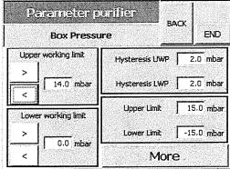
Using the foot pedal control, adjust the gas pressure inside the box until the pressure reaches the desired level range.
