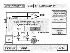
Using the regulator, turn on the regeneration gas supply and set the pressure to 5psi.
