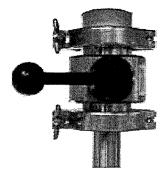
Refill the antechamber by turning the refill valve to the **open** position.
