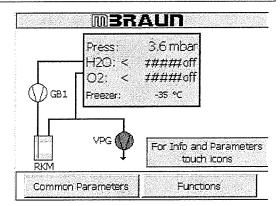
Use the arrows listed under Upper Working Limit and Lower Working Limit to increase or decrease the box atmosphere pressure setpoint in one tenth decimal intervals.
