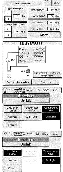
The glovebox will continue to circulate the working gas until the function is deactivated.
