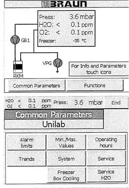
Touch the Freezer/Box Cooling button on the parameters screen to display the Freezer/Box Cooling parameters screen.
