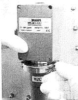
Insert the analyzer cable plug into the hole on the analyzer by pushing the plug into the hole gently until it snaps into place.
