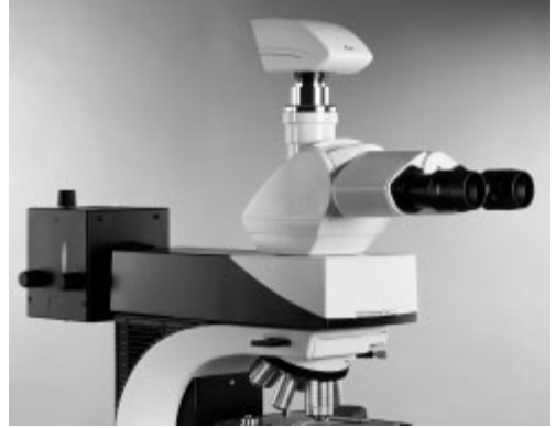
Fig. 20 Mounting the 106 z lamp housing 1 Lamp housing receptacle
