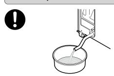
Insert the attached drain hose in the drain water port and drain water at least 2 hours after operation. If water is drained out in haste, hot water may splatter, resulting in burns or damage to the floor.Repeated use of the same heating water may corrode the chamber or clog the piping.
