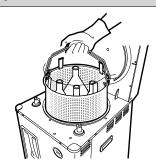
Be sure to wear thermally insulated leather gloves. Note that it takes time until liquid is cooled down. Handling a sterilized object with bare bands immediately after the end of operation may result in burns.
