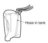
Be sure to insert the hose in the tank into the holes at the back inside the exhaust tank.
