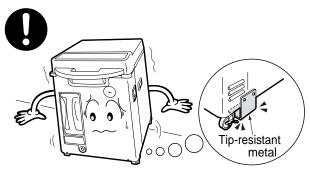
Anchor the product firmly with the tip-resistant metal attached to the product.
