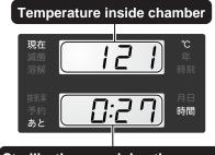
Sterilization remaining time or melting remaining time (after the temperature reaches the sterilization temperature or melting temperature)
