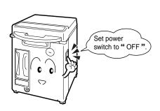
Set the power switch to "OFF" and sufficiently cool the product before performing maintenance. Failure to observe this warning may result in electric shock or burns.
