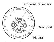
(Plan of bottom of chamber inside)
